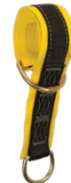
PASS-THROUGH CHOKER ANCHOR Features 1-3/4" load-bearing web with 3" wide full-length wear pad for abrasion resistance. Appropriately sized alloy steel D-rings provide simple pass-through choke-on installation. Sizes: 3',6',8',10',12'
