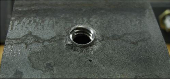
Material rolls in to fill space, increasing thread engagement.
