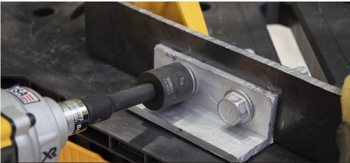
Install with impact wrench and impact ready socket driver.
